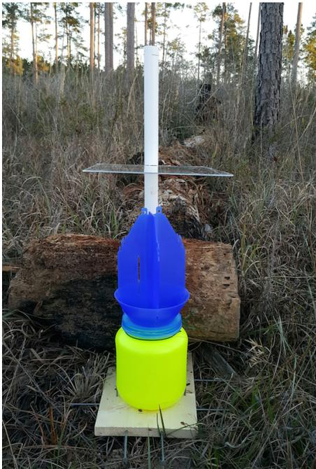
Fig. 2. Blue vane trap.
